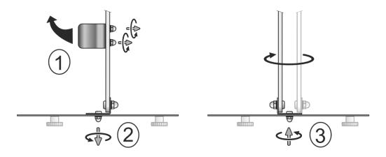
fasten the Wx8xx transmitter (with the SP015C Batteries holder connected) with two M4 screws to the shield mounting bracket as shown. Longer screws are included in the SP015C delivery. The mounting bracket and both devices should now be exactly on the center axis of the shield interior space.
