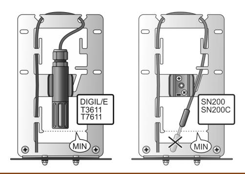
If the probe cable is too thin (approx. 2 to 3 mm, eg for the TG3 probe) and there is a risk of instability of the probe sensor, secure the probe cable by turning the probe holder. See pictures below.
